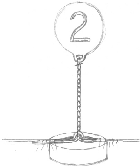
Figure 3G - Diagram showing the Dive Trail sinkers and line
