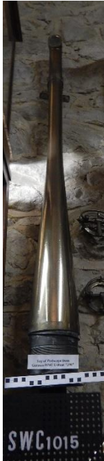
Figure 51: Navigating (aft) periscope upper section
