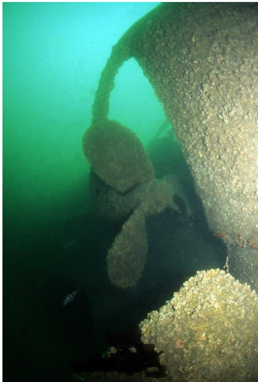
Figure 17: Port propeller (note the missing cone) and aft hydroplane. Bottom right: the lower leading edge of the rudder can be seen.
