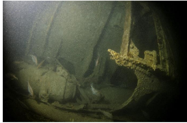
Figure 27: Pressure hull, outer casing and HP cylinder.
